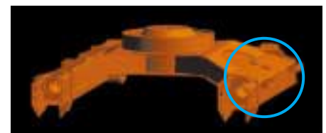
Undercarriage Designed for Easy Mud Removal
